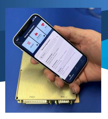
The unprecedented flexibility afforded by the ap allows the audio systems to be configured easily for different mission profiles. This is very useful when an aircraft is leased for multiple uses such as forestry and medivac. Access to the configuration mode is limited to line installer/maintenance personnel, who must be within 1 meter of the LRU, and initialize the mode from the unit itself.
