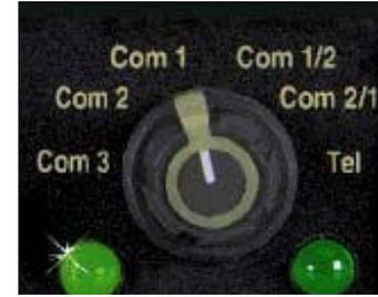
When the mic selector switch is in the **Com 1** position, both pilot and copilot will be connected to the Com 1 transceiver. Only the person who presses their Push To Talk (PTT), will be heard over the aircraft radio. Turning the rotary switch to the COM 2 position will place pilot and copilot on Com 2.
