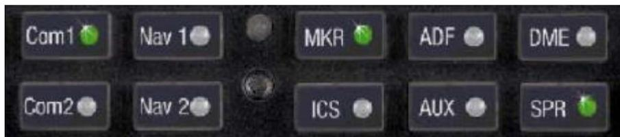
Because the rotary microphone selector switch controls what transceiver is being heard, the **Com 1** and **Com 2** push-buttons are of the momentary type and do not remain in when selected. This is also part of the "auto" function. You will always hear the audio from the transceiver that is selected for transmit by the rotary mic selector switch.
