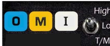
The Blue lamp, labeled "O," is the Outer Marker lamp and has an associated 400-Hertz 'dash' tone. The lamp and tone will be keyed at a rate of two tones/ashes per second when the aircraft is in the range of the Outer Marker Beacon.
