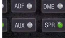
Unswitched audio, (autopilot disconnect, altimeter warning, etc.) will come through the speaker regardless of the speaker button position.
