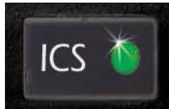
The front panel ICS switch controls muting of entertainment source #1 (for pilot and copilot). Pushing this button places the ICS in Karaoke (or sing along) mode, which inhibits the soft mute feature. This allows the music to continue uninterrupted by intercom or radio traffic when cockpit workload is appropriate.
