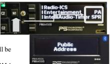
To exit PA mode, push and hold the **N1** button again until **PA** is off or cycle power on the audio panel.
