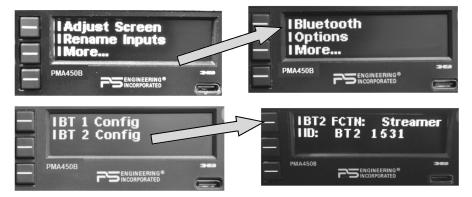
To pair the PMA450B PS Streamer with a compatible device, access the streamer menu from Radio-ICS  $\rightarrow$  More  $\rightarrow$  Streamer  $\rightarrow$  Config  $\rightarrow$  Pair. Now, turn on the desired device and initiate the pairing on the device as well.
