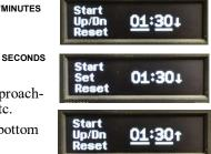
Press the SET button and adjust the desired time
