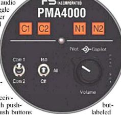
$N1\ ({\rm Nav}\ 1),\ N2\ ({\rm Nav}\ 2)$  are "latched" type switches. When one of these buttons is pressed, it will stay in the "in" position. Press the switch again and it be in the "out" position and remove that receiver from the audio. While selected, an internal lamp will also annunciate the switch.
