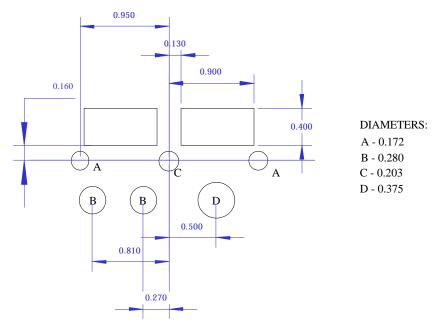
Figure 6-1- Hole Configuration
