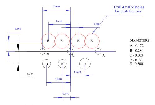
Figure 6-2 Hole Configuration to avoid rectangular cutouts
