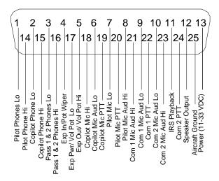
Figure 6-3 Connector Layout
