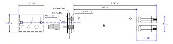
Figure 6-4 Installation Diagram
