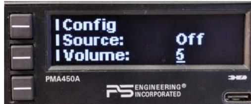
From the PS Streamer menu, push the middle line select button to toggle between communication radio audio and all audio heard in the pilot headset, including radio, intercom, music and telephone.
