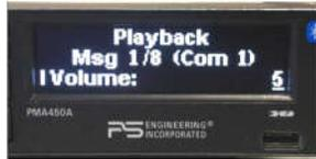
To play back the last recorded message, press and hold the COM Receive pushbutton associated with the selected radio transmitter. You can either wait for the message to finish playing before accessing the prior message, or cancel the current playback and step backward. To cancel the playback, press and hold the
