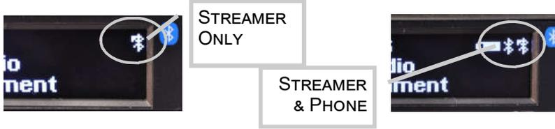
The PS Streamer defaults to “off” when the audio panel is turned on each time. You will need to activate the PS Streamer for each flight when desired, but pairing will not be necessary. The module will reconnect when activated.
