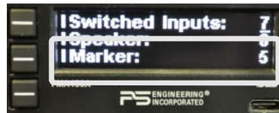
Marker Beacon sensitivity is changed from Low to High sensitivity by pressing and holding the **MKR** button for 2 seconds, or until "**H**" appears in the display, indicating High sensitivity is activated.
