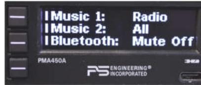
In addition to the panel mute menu, a remote switch may be installed to allow the passengers local access to their Mute Off mode. When this switch is grounded, the menu choice is overridden.
