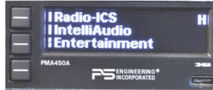
Non-voice signals are blocked. When someone speaks, only their microphone circuit opens, placing their voice on the intercom.
