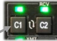
COM receive button for two seconds. The next time the button is pressed for one second the next earlier message is received. The screen displays a status message to indicate that playback is in progress. The playback will stop whenever there is more incoming selected COM audio, and the message can be replayed from the beginning by pressing the selected COM receive button again.
