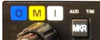
The White lamp, labeled "I", is the Inner marker and has a 3000 Hertz 'dot' tone. The lamp and tone will be keyed at a rate of six times per second.
