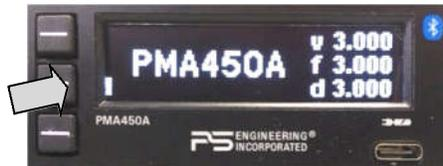
During the unit boot up process, press the lower line select button until the setup screen appears. This will place the unit into the “User Configurable Mode- home screen”. This allows adjustment for:
