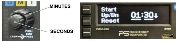
The set time is remembered until changes, and can be reset to the last value. The count up timer simply shows elapsed time since START, and counts to 99 minutes, 99 seconds.
