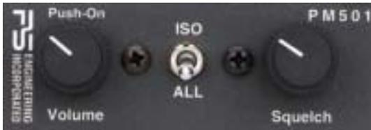
The PM501 has an automatic, fail-safe connection to the aircraft radio. In the event that power to the intercom is lost, an internal relay will immediately connect the pilot's headset directly to the aircraft radio.
