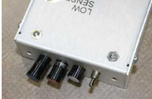
Figure 2-3 - MB10 with lamps extended for installation
