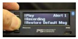
Hold the center button to record a new message using the pilot's microphone Pressing the bottom button will replace the user-stored message with the factory message. In the case of Alert 1, it is a simple chime sound.
