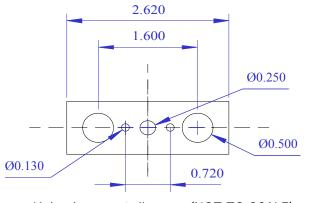
Hole placement diagram (NOT TO SCALE)
