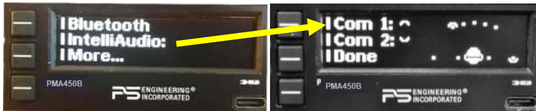
Figure 3-14 IntelliAudio – True Dimensional Sound, Spatial Location Display, showing C1 at 30° left and C2 at 90° right of center.
