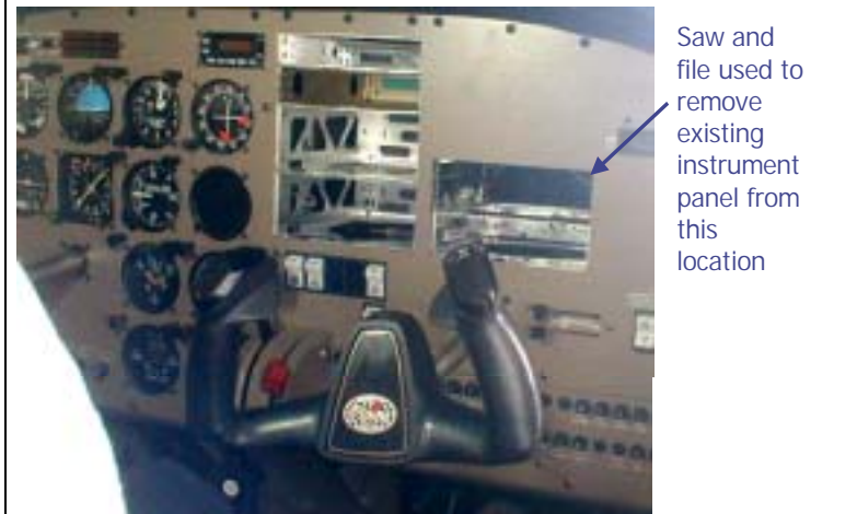
Figure 2-3 Completed panel opening (Typical)
