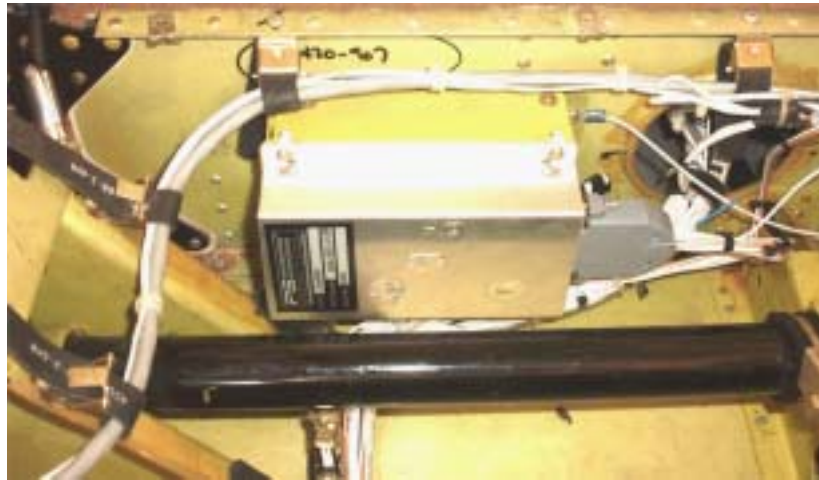
Figure 2-9 View of typical PVA802 Installation
