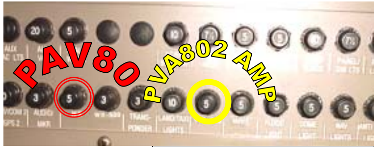
Figure 2-8 PVA802 Dist. Amp Circuit breaker location (Typical)
