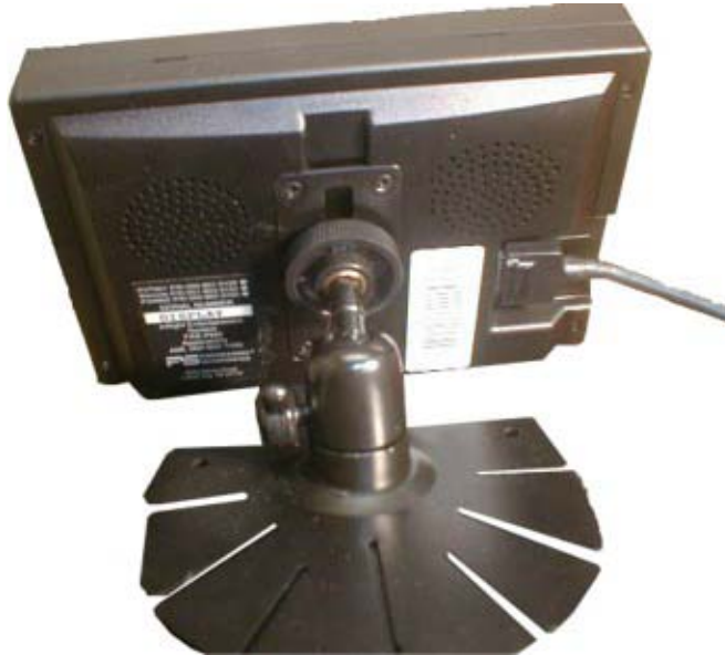
Figure 2-8 Portable mounting bracket with PVA801 attached
