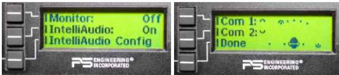
Figure 3-3 IntelliAudio – True Dimensional Sound, Spatial Location Display, showing C1 at 30°left and C2 at 90° right of center.
