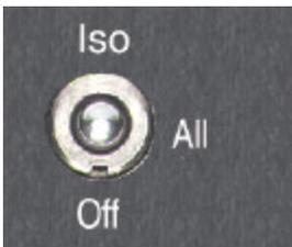
Unit power is turned on and off by the mode selector switch. In the OFF or "FAIL-SAFE" position, the pilot is connected directly to Com 1 allowing transmit and receive capability regardless of unit condition. Any time power is removed or turned OFF, the audio selector will be placed in the fail-safe mode. The switch is a 3-position mode switch that allows the pilot to tailor the intercom function to best meet the situation.
