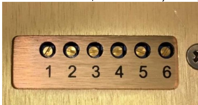
Figure 2-3— Adjustment potentiometers (NOTE these are all 30-Turn pots, and may require 10-15 turns to notice any change)
