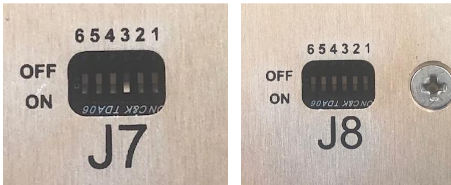
Figure 2-4 LOGIC SWITCH LOCATIONS PAC45J
